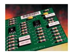
Extreme temperature and environmental durability is achieved with polyimide labels, perfect for bar coding or labeling PC boards and other electronic components.
