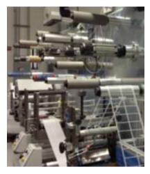
Servo-driven, precision diecutting, with tolerances as tight as  $\pm 0.001''$  when using flat bed dies.
