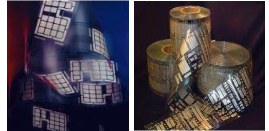
Screen printed flexible circuitry delivered on rolls allows for high volume production at a lower cost.
