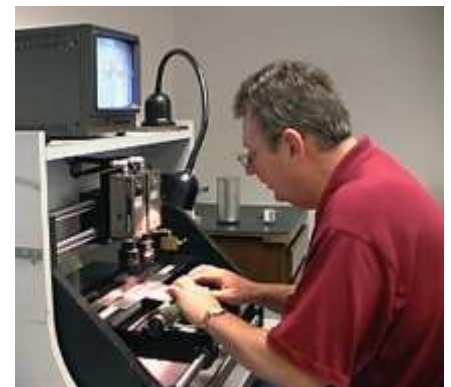
An advanced video plate mounting system ensures print registration and consistency throughout a production run.
