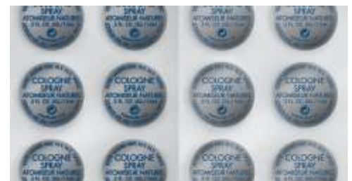
These samples (analog plate printing on the left, digital plate printing on the right) demonstrate the superior print quality digital plates afford.
