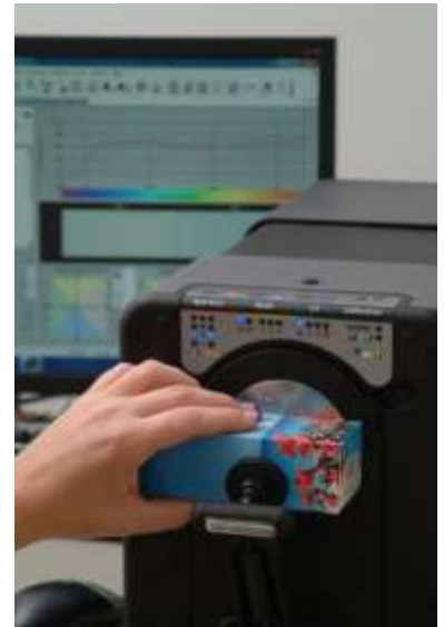
A computerized spectrophotometer digitally scans color data to evaluate every color match we produce.
